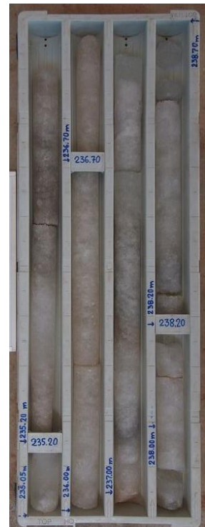
Core tray from RZK-01A containing Carnallite
