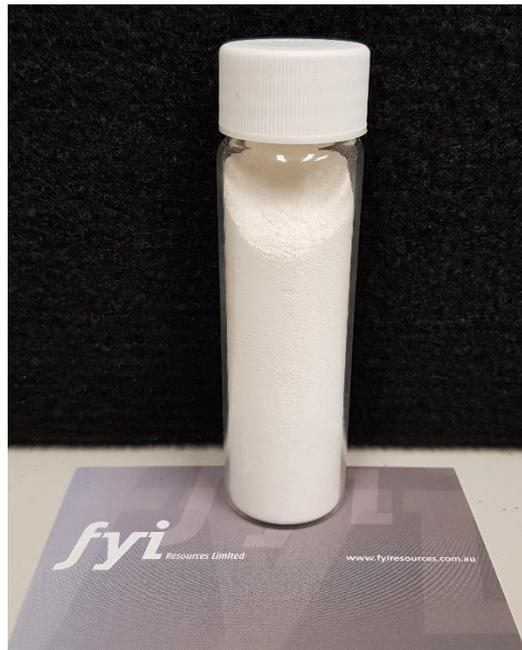
***FYI's HPA produced from Cadoux kaolin feedstock (99.997% Al<sub>2</sub>O<sub>3</sub>)***
