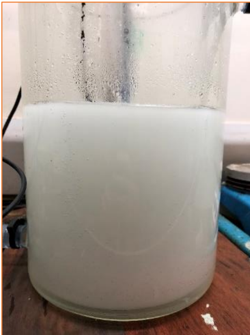
Images of FYI Resources 99.999% (5N) high purity alumina at final stage of precipitation at laboratory
