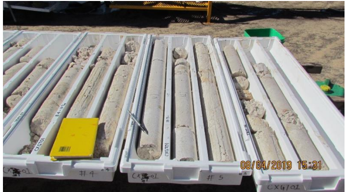
Diamond drill core from Cadoux kaolin project April 2019
