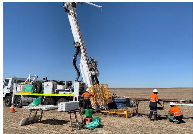
Diamond drilling at Cadoux kaolin project April 2019
