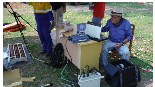
Calibrating the down-hole geophysics equipment at the Sino-Lao Potash project
