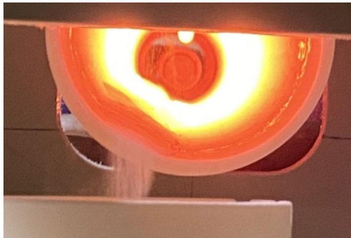
Figure 1: FYI Resources Continuous Furnace in Operation
